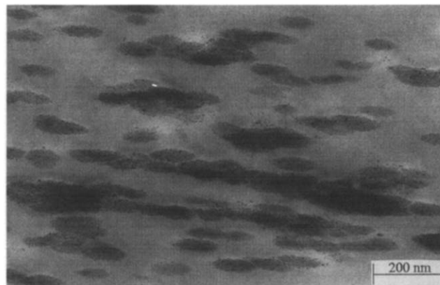
Figure 9 Transmission electron micrograph of a PVC/MBS blend with a SBR particle size of 82 nm (MBS, AGGL type), deformed in uniaxial tension
